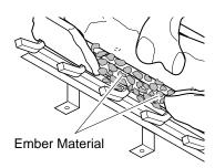
Figure 55 - Placing Ember Material on Burner
